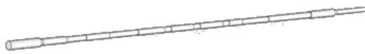
图 7 二次优化后的超声刀模型示意图 Fig.7 Schematic of the ultrasonic scalpel's model after quadratic optimization
