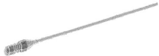
图 2 连接有换能器的手术刀模型示意图 Fig.2 Model of ultrasonic scalpel with transducer
