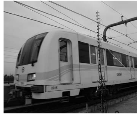
图 2 列车噪声测试实景图 Fig.2 The linear microphone array for measuring pass-by noise
