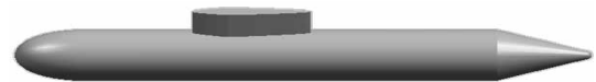
图 9 复杂线形长柱壳模型 Fig.9 Model of a complex slender cylindrical shell
