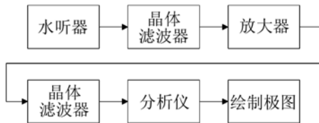
图 2 常规参量接收阵系统框图 Fig.2 Diagram of a regular PARRAY system
