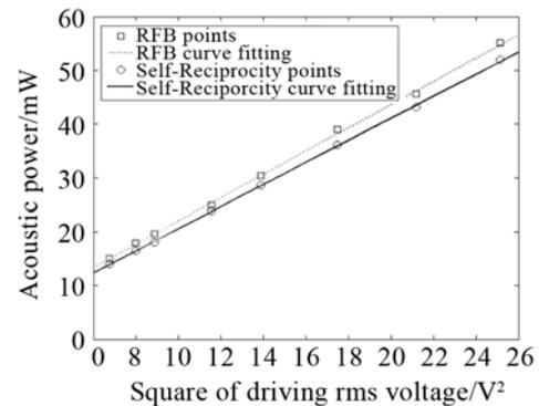
Fig.5 Measurement result of output power vs. exciting RMS voltage squared for 15MHz focusing transducer (OlympusV319, SN 76 3322) with backing ,normal aperture: 0.5 inch, normal focal length: 60 mm
