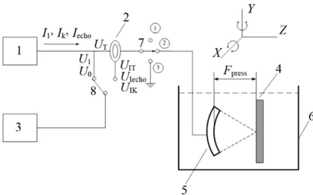
Fig.3 Scheme of free field self-reciprocity calibration apparatus 1-tone burst generator; 2- current monitor; 3- oscilloscope; 4- reflector; 5- focusing transducer; 6- water tank; 7- three-way switch for open circuit/work load/short circuit of the generator; 8- two-way switch for voltage/current signal detection
