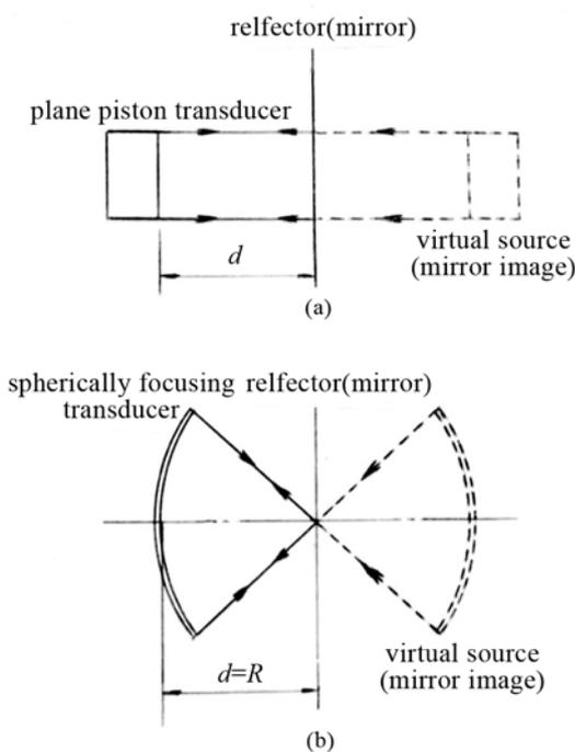
Fig.1 The ideal scheme of the self-reciprocity method for plane piston transducer (a) and spherically focusing transducer (b)
