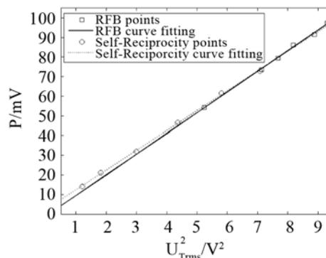
**Fig.6 Measurement result of output power vs. exciting RMS voltage squared for 10MHz focusing transducer (air backing)**
