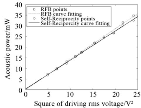
Fig.4 Measurement result of output power vs. exciting RMS voltage squared for 5 MHz focusing transducer(Olympus V308, SN 763325)
