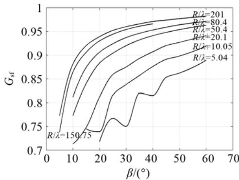
**Fig.2** The diffraction correction coefficient  $G_{\text{sf}}(R/\lambda, \beta)$  of spherically focusing transducer in self-reciprocity calibration vs. focus half-angle  $\beta$  and the ratio  $R/\lambda$  of the curvature radius  $R$  to wave-length  $\lambda$  where  $R=F_{\text{pres}}$ , the pressure focal length
