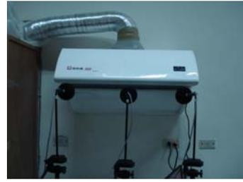
Fig.3 Locations for noise measurement by sound level meters
