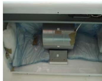
Fig.17 Absorption glasswool packed by PU film
