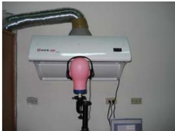
Fig. 2 Artificial head and torso simulator
