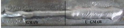
图 13 滴状过渡焊道外观对比(右侧施加超声) Fig.13 Weld appearances of MIG and U-MIG
