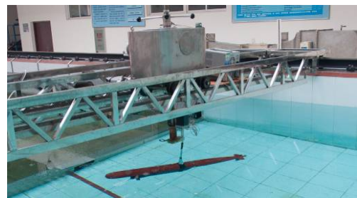
图 10 距离像测量实验环境 Fig.10 Experiment environment for range profile measurement
