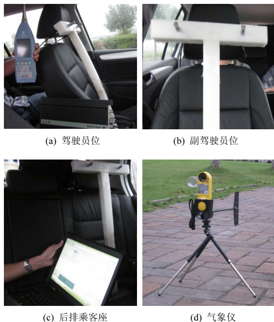
图 1 车内噪声测量中设备的设置 Fig.1 The setting of interior noise acquisition in measurement
