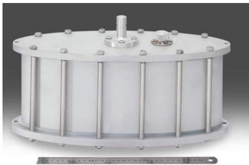
图 11 稀土 IV 型弯张换能器样机 Fig.11 The prototype of the class IV rare-earth flextensional transducer
