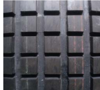
图 10 等节距花纹轮胎 Fig.10 Equal pitch tires
