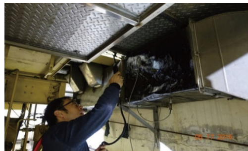
图 9 利用声强计测量通风管道壁面的声强 Fig.9 Measurement of sound intensity of ventilation duct by sound intensity probe
