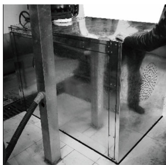
图 10 改造前安装隔声罩的电动机 Fig.10 Motor with soundproof cover before transformation
