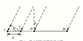
图 1 基元间隔相等的线列阵 Fig.1 A linear array of equally spaced elements
